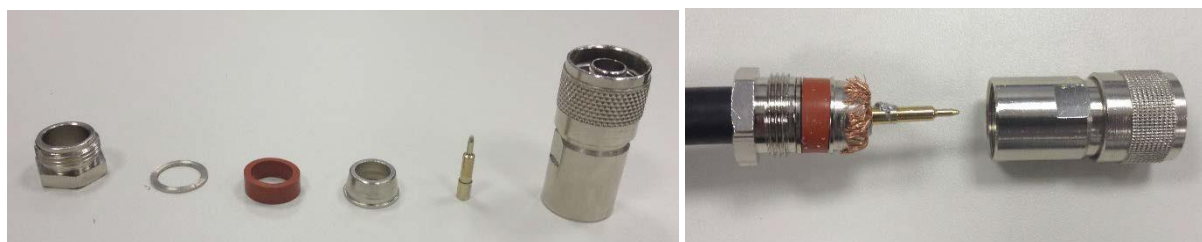
Parts of N-type connectors
